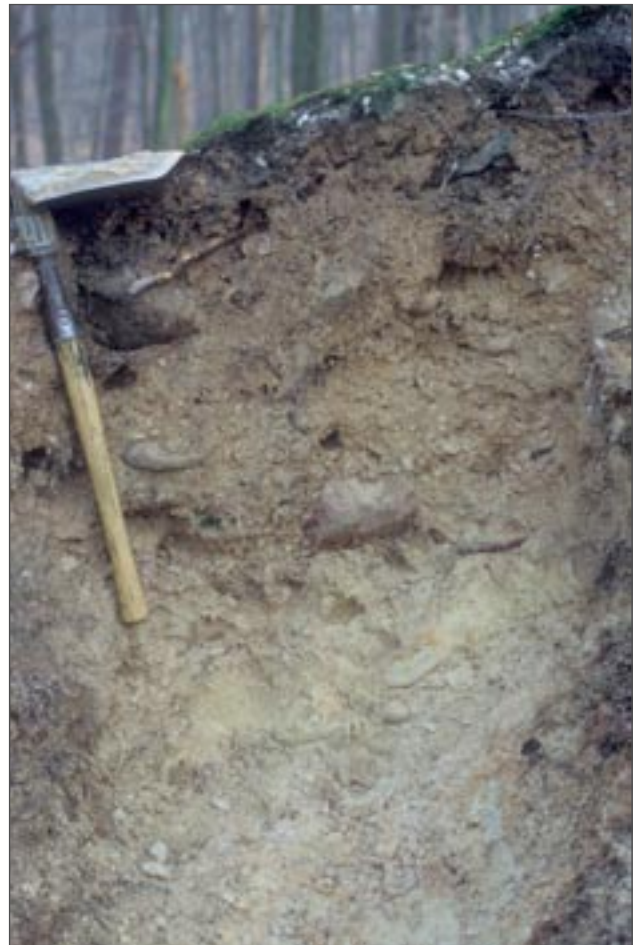
Photo 1 Upper slope layer in top of Devonian slates (Taunus Moutain) Explanation in text and under photo 2
