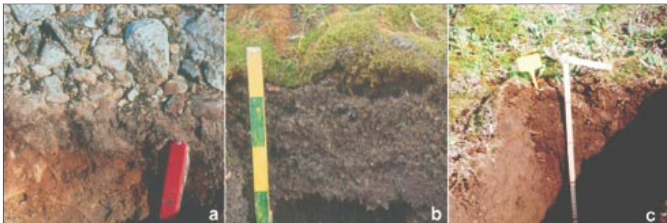
Figure 1. Representative sites with permafrost; (a) Lepti-gelic Podzol (C3); (b) Dystri-gelic Fluvisol (A4); (c) Molliturbic Cryosol (B1)
