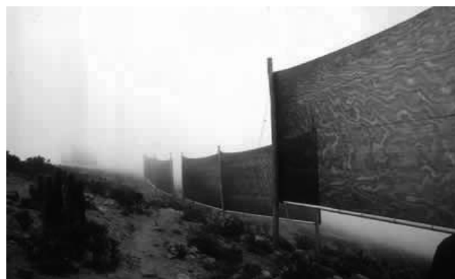
Fot. 2. Kolektor pasywny do poboru prób osadów mgielnych (Chile) ( www.fogquest.org ) Photo 2. Passive collector to collecting cloud/fog water (Chile) ( www.fogquest.org )
