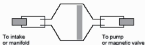
Ryc. 3a. Banieczka z filtrem ceramicznym do dwutlenku azotu (3) Fig. 3a. Sintered glass filter in a glass bulb for \text{NO}_2 sampling (3)
